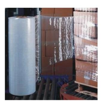
A highly stretchable plastic film commonly made from Linear low-density polyethylene (LLDPE) wrapped around items. The elastic recovery keeps the products tightly bound.
